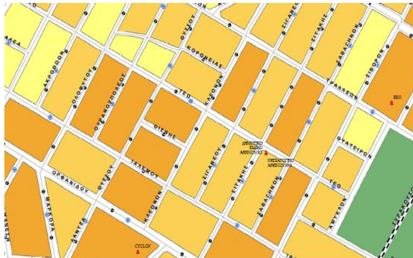
Figure 1: Sample solution. The blue and black dots refer to blue and common containers, respectively. The tension of the colour of each block is analogous to population density. Dark orange colours indicate dense populated blocks, while light yellow colours indicate sparse populated blocks. The red marks indicate points of interest.
